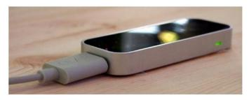
Fig. 2. Leap motion controller
